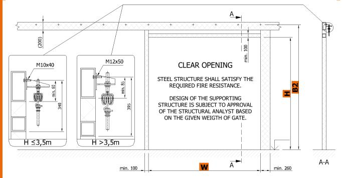
Construction readiness of the opening is secured by the customer according to the requirements of the contractor and depending on the type of jamb and lintel of the opening.
