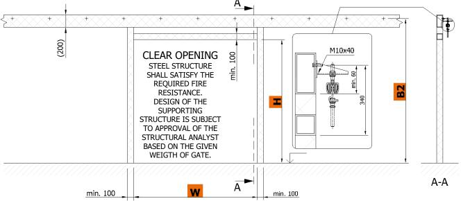
Construction readiness of the opening is secured by the customer according to the requirements of the contractor and depending on the type of jamb and lintel of the opening.
