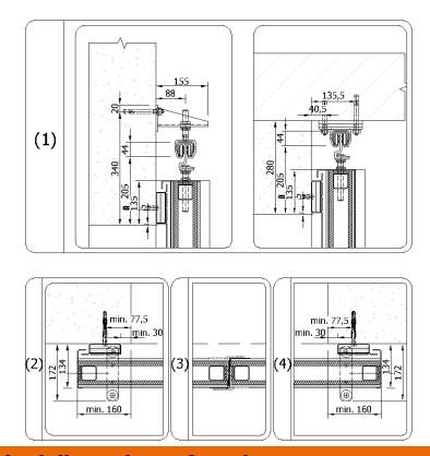
Minimum required dimensions of steel structure
