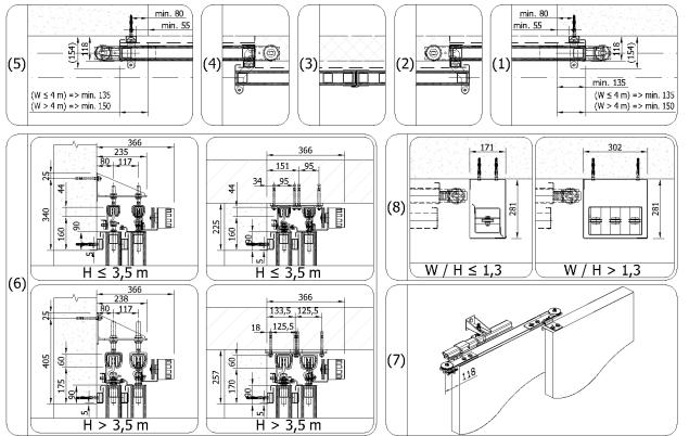
Minimum required dimensions of steel structure
