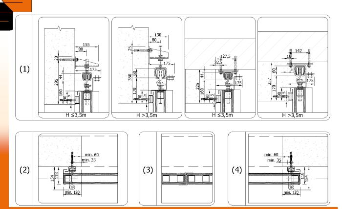
**Minimum required dimensions of steel structure**
