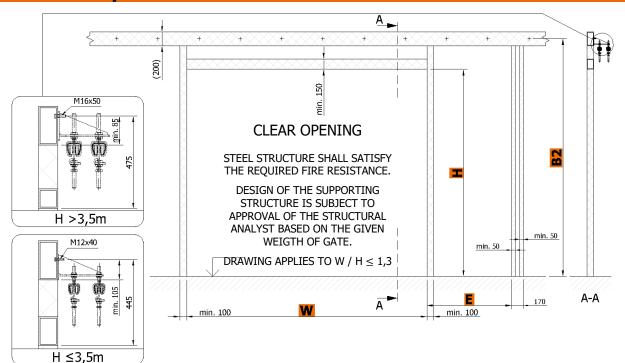
Construction readiness of the opening is secured by the customer according to the requirements of the contractor and depending on the type of jamb and lintel of the opening.
