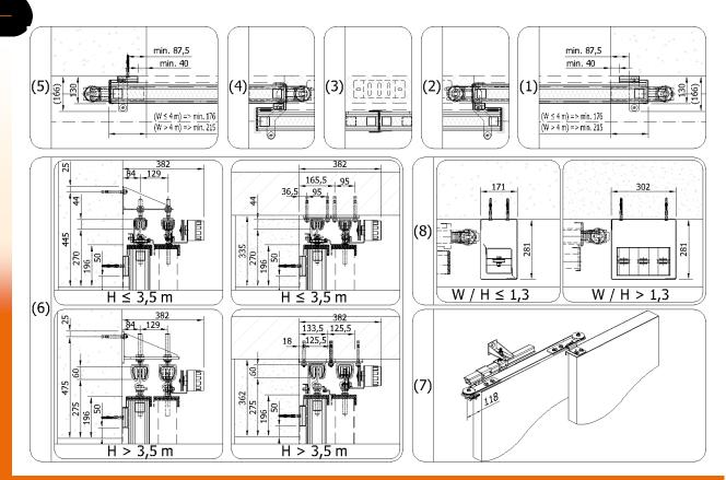
Minimum required dimensions of steel structure
