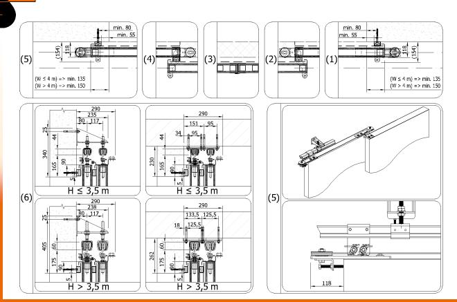
Minimum required dimensions of steel structure
