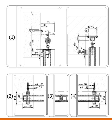
Minimum required dimensions of steel structure
