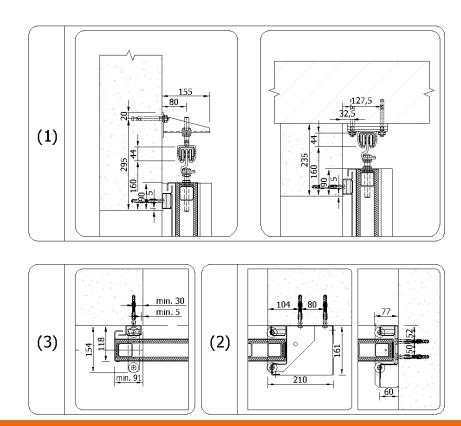
**Minimum required dimensions of steel structure**
