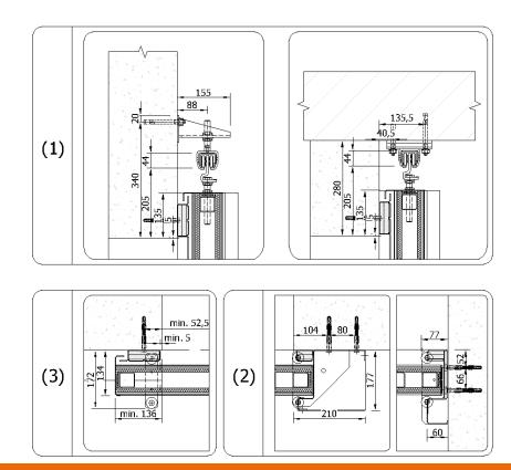
**Minimum required dimensions of steel structure**
