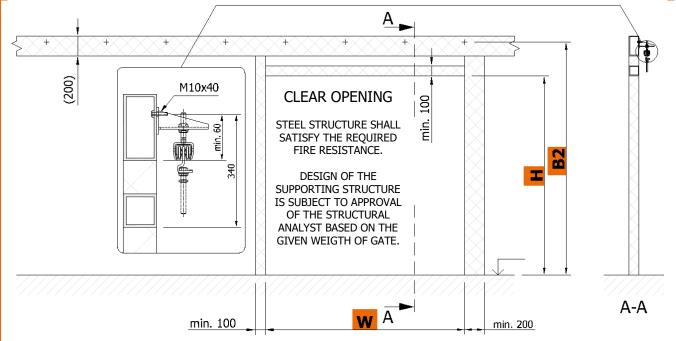
Construction readiness of the opening is secured by the customer according to the requirements of the contractor and depending on the type of jamb and lintel of the opening.
