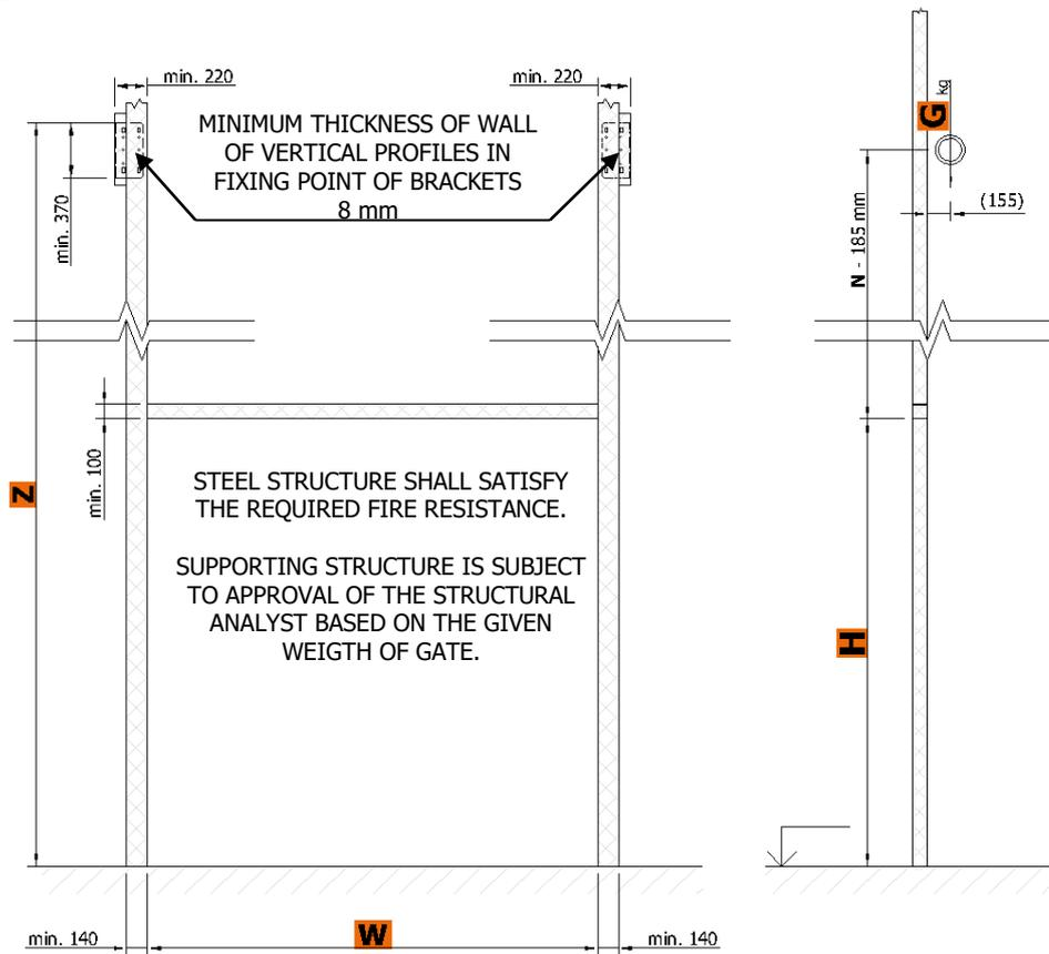
Construction readiness of the opening is secured by the customer according to the requirements of the contractor and depending on the type of jamb and lintel of the opening.
